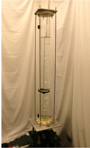
Figure 3-4. Bubble column mounted on the shaker table via vertical beams (threaded rods).
