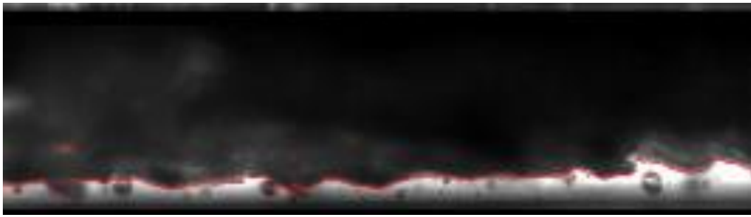
Figure 2-17. Processed PLIF image of vertical annular flow; U_{SG} = 55.3\text{m/s} , U_{SL} = 0.127\text{m/s} , D = 23.4\text{mm} (adapted from Schubring & Shedd, 2008).
