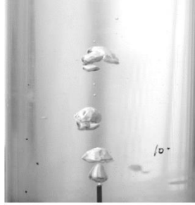
Figure 3-7. Single point injection of air inside of the column ( D = 102\text{mm} , d_{inj} = 1.6\text{mm} at 90^\circ , and U_{SG} = 6.9\text{mm/s} at P_m = 600\text{ kPa} ).
