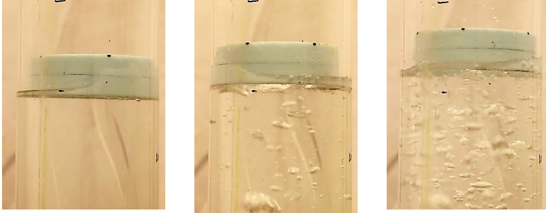
Figure 3-13. Void fraction measurement using surface displacement from tracking the Styrofoam at U_{SG} of (a) 0, (b) 4mm/s, and (c) 10mm/s
