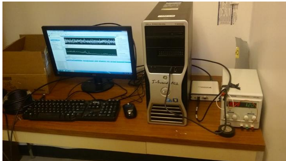
Figure 15: Data acquisition system for Fab Lab roof top deployment including the DC power supply, digital signal analyzer, and computer.
