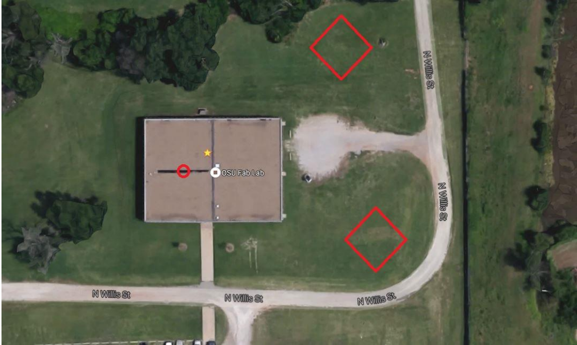
Figure 18: Locations of microphone deployments at the OSU Fabrication Laboratory. The red circle denotes the location of the current roof top microphone, and the diamonds represent the planned locations of the 2 nd and 3 rd microphones assemblies.
