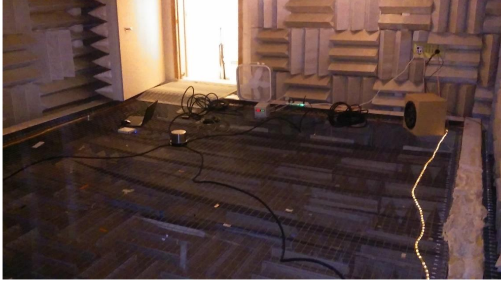
Figure 31: Infrasonic setup inside of anechoic chamber with soaker hoses attached to the Chaparral microphone, subwoofer, and the box fan.
