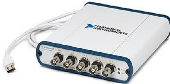
Figure 13: National Instruments image of their NI USB-4432, which is used to acquire the signals from the Chaparral microphones.
