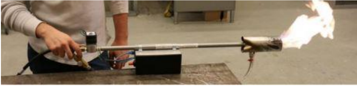
Figure 24: Pulsed gas-combustion torch in operation at the Fab Lab.
