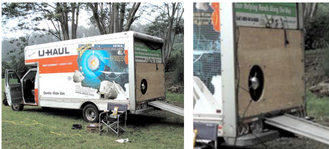
Figure 3: (left) Picture from Park & Robertson (2009) of the TRW mounted on the side of a moving truck to make it portable. (right) Same picture zoomed in on the TRW.
