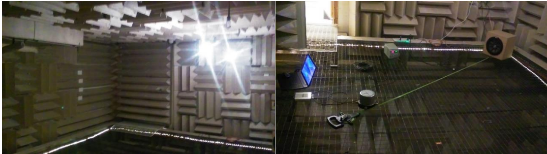
Figure 28: Oklahoma State University anechoic chamber (left) before the experiment was set up and (right) during testing.
