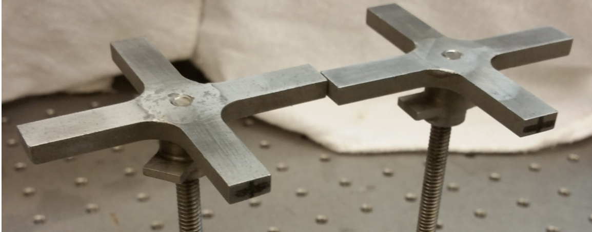
Figure 2.7: Final test model configurations: out-of-phase scissor links (left) and in-phase scissor links (right).
