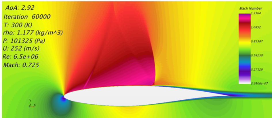
Figure 6.3: Mach profile indicated that small scale backward-facing steps in transonic flows may produce additional shock features and influence aerodynamic properties.
