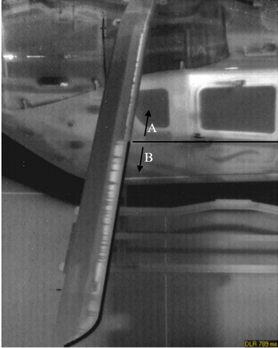
Figure 1.1: Transition on inboard section of rotor blade (“A”), where 0.367 mm protective tape is applied, is shown to occur prior to thirty percent chord. This early transition is not ideal, and highlights the drawback to leading edge protective tapes and to backward-facing steps in aerodynamic flows. The outboard section of the rotor blade (“B”) is utilizing an embedded leading edge protection, which produces a smaller step height [7].
