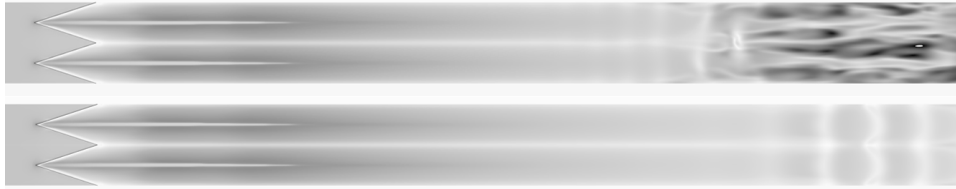
Figure 5.28: Comparison of phase 2 refined mesh with half sized and original sized domain; notice downstream effect.
