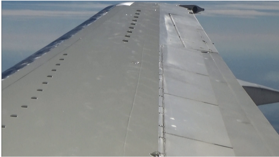
Figure 4.2: Example of shock wave visualization over wing during baseline fuel consumption flights.
