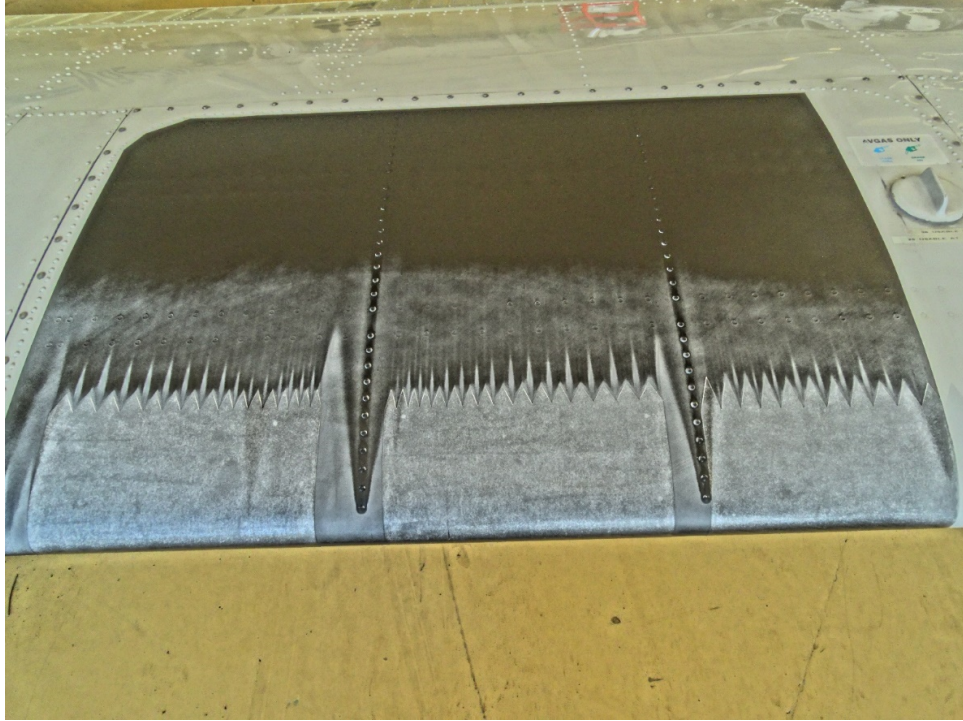
Figure 4.4: Results of wall shear stress flight testing by Edge Aerodynamix.
