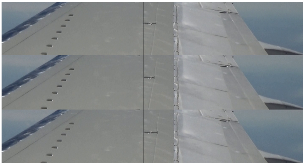
Figure 4.3: Example of shock instability over 0.3 seconds during baseline fuel consumption flights without the CVG installed.
