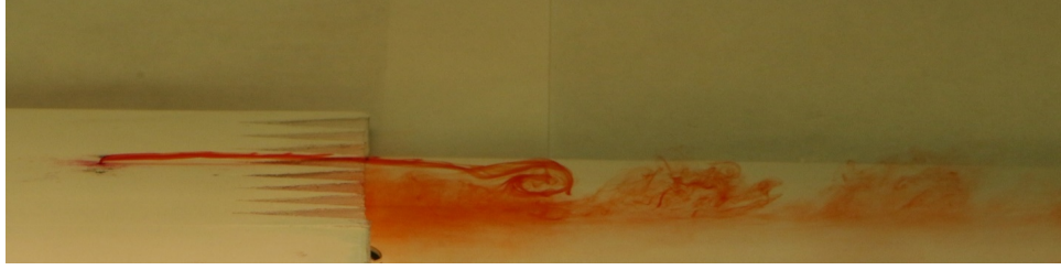
Figure 5.13: OSU water tunnel dye flow visualization over 1.0 cm CVG step at 10 m/s. The four flow structures associated with backward-facing steps are shown (shear layer, recirculation, rollup, shedding).
