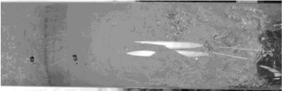
Figure 5.19: Submerged float during test at f = 15 Hz, A = 6.5 mm, U_{SG} = 5.0 mm/s
