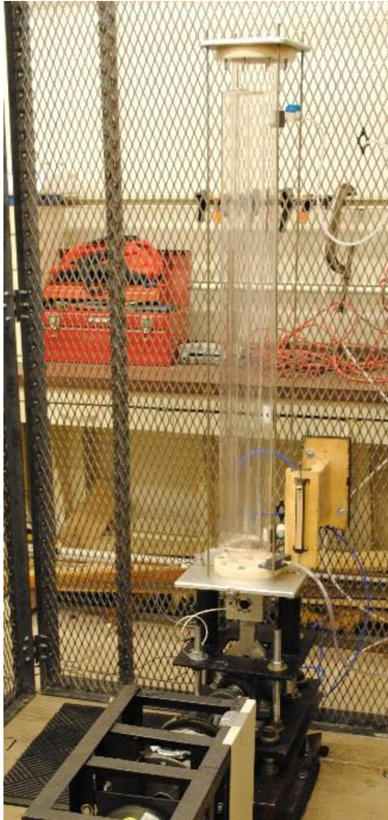
Figure 3.29: Final constructed shaker design with test column
