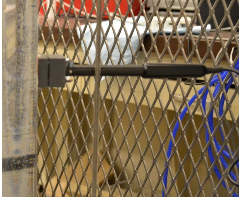
Figure 3.5: DO probe installed on the cylinder
