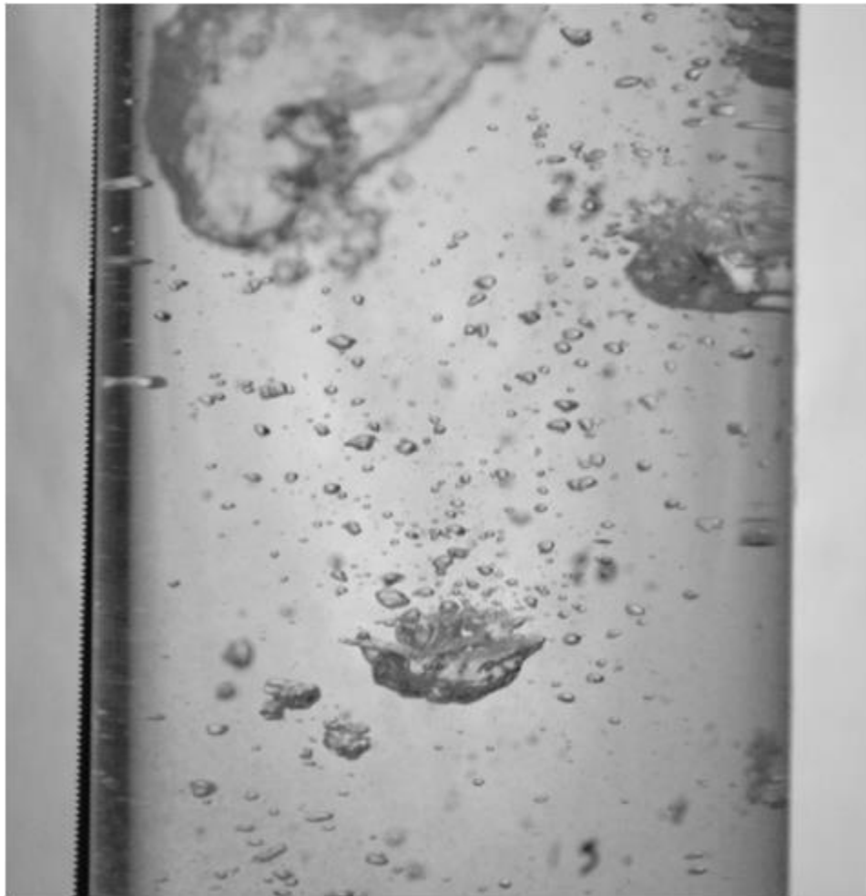
Figure 6.1: Photograph of bubble breakage phenomena in vibrating BCR
