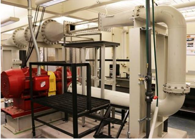
**Figure 3. Completed water tunnel installed at Oklahoma State University in the Experimental Flow Physics Lab.**
